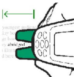
7. Glide the Pen from right to left in a straight line over the text. Start scanning 1cm from the end of the text and finish 1cm after the beginning of the text.
