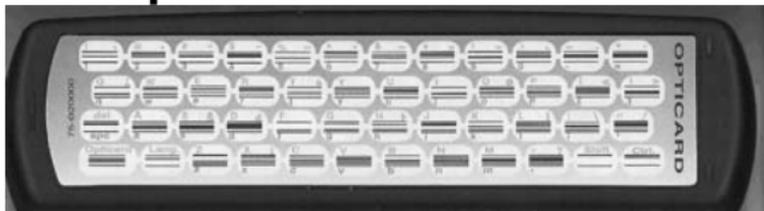
The **Opticard** is a scanning keyboard found on the back of the Pen case.
