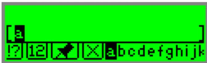
Use the **Character Bar** to manually insert or edit text. The **Character Bar** is only available when the Pen is in **Edit Mode**. Scroll to the field you wish to edit and press ENT to activate **Edit Mode**.
